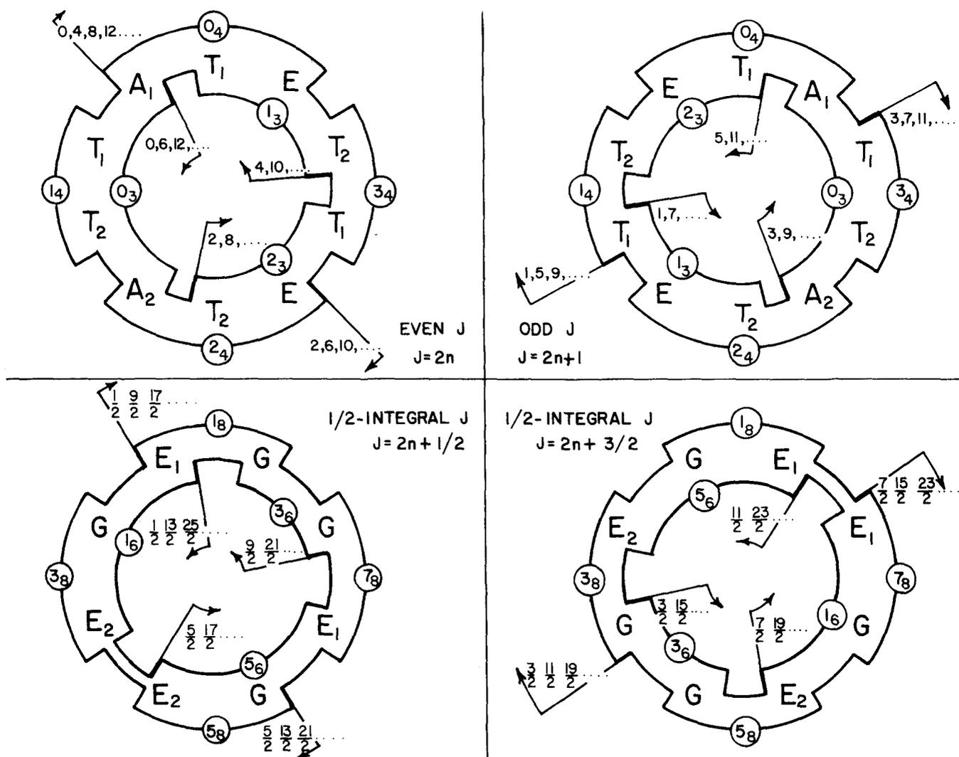
FIG. 7. Progression of cubic IR in the spectrum of lowest order hamiltonian. The diagrams give the ordering of the cubic IRR in a  $J$ -manifold spectrum due to a potential of the form  $(x^4 + y^4 + z^4)$  for any  $J$ . Level clusters are indicated by blocks labeled by cluster numbers in circles.
