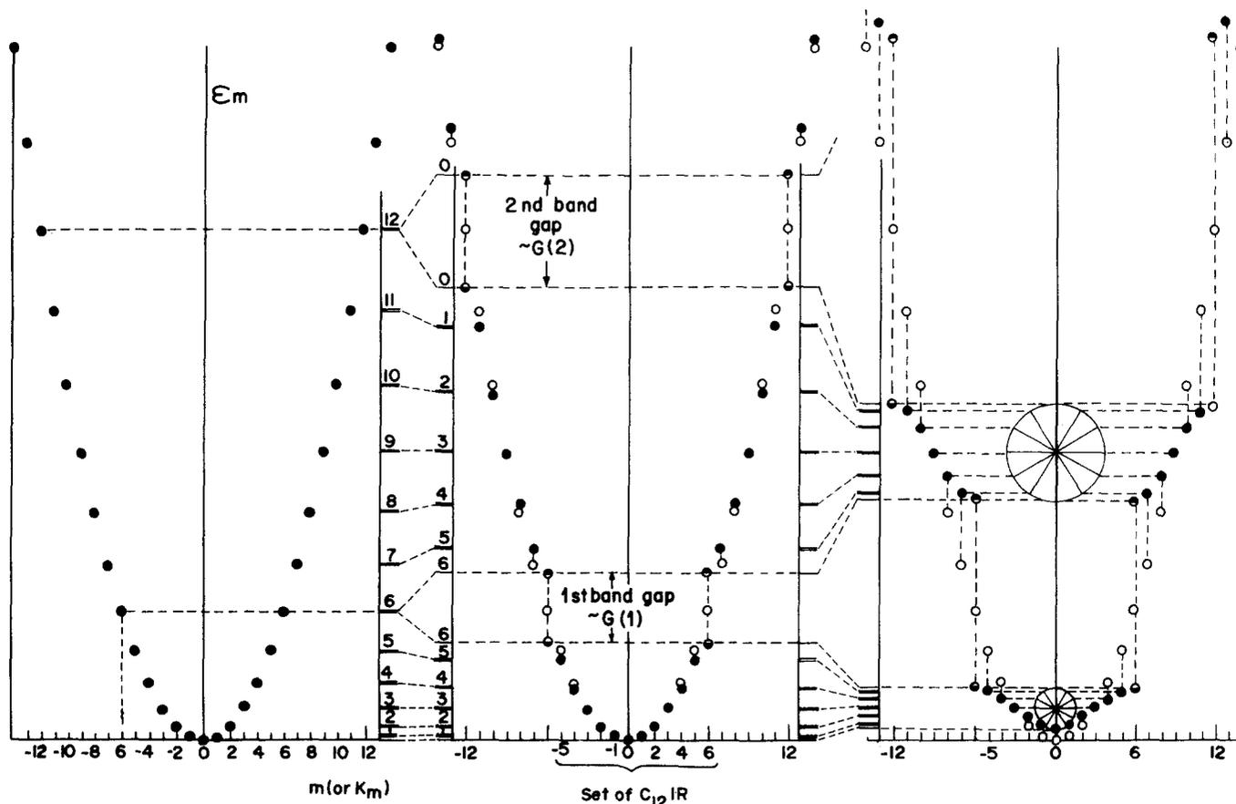
FIG. 1. Eigenvalue spectrum of a one-dimensional periodic potential ( $D_{12}$  Symmetry). (a) Zero potential. (b) Weak potential. (c) Strong potential.
