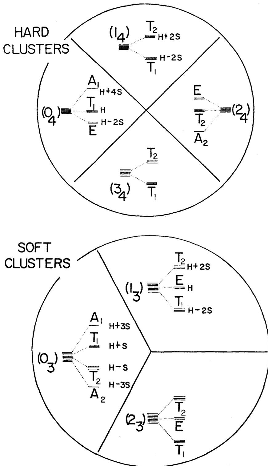
FIG. 6. Octahedral cluster splitting patterns. If only nearest neighbor tunneling amplitudes  $S_m = S$  are assumed nonzero in the energy equations [Eqs. (III. 20b)–(III. 22b)] then they predict the form of splitting shown here.
