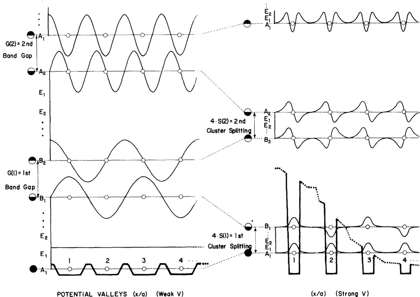
FIG. 2. (A, B)-standing wave solutions to one-dimensional periodic potential ( $E$ -waves are not drawn.) (a) Weak potential. Energy differences are determined by potential energy only to zeroth order. Waves which hover over the potential hills are higher in total energy. (b) Strong potential. Energy differences are determined by the number of zeros or nodes in the wave. Waves with more nodes are higher in total energy even if the nodes fall in the center of potential hills.
