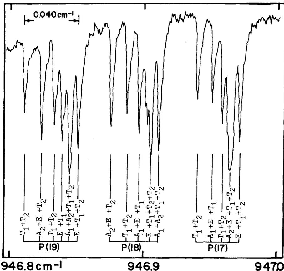
FIG. 5. Tunable laser diode absorption spectra of SF<sub>6</sub>. [after J. P. Aldridge, H. Filip, H. Flicker, R. F. Holland, R. S. McDowell and N. G. Nerson, *J. Mol. Spectrosc.* 58, 167 (1975).]
